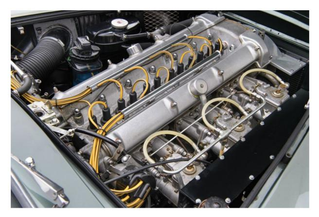
The DB4GT, with its higher compression ratio of 9:1, larger inlet and exhaust valves, and uprated camshafts, had a claimed output of 302 bhp at 6,000 rpm. The DB4GT could reach 60 mph in just over six seconds, and a quarter of a mile distance reached from a standing start in 14 seconds, hitting a speed of 98 mph. The top speed was just over 150 mph.
